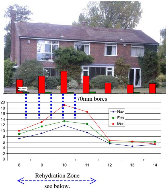
Douglas Pierie, the surveyor appointed by the school to advise on the subsidence that has taken place, arranged for the Wisteria to be cut back and adjoining shrubbery to be removed in February. In addition, he sank 70mm dia. bores at 1m ctrs along the left one-third of the rear elevation (see above and plan on last page) and the school arranged for them to be topped up with water.
