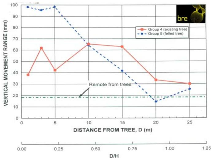
Interestingly, for both sets of rods, the greatest movements do not appear to occur at the point nearest the tree, but a few metres away. This is particularly noticeable for the rods emanating from the existing tree, where maximum magnitude of movement has occurred some 10m away from the tree.
