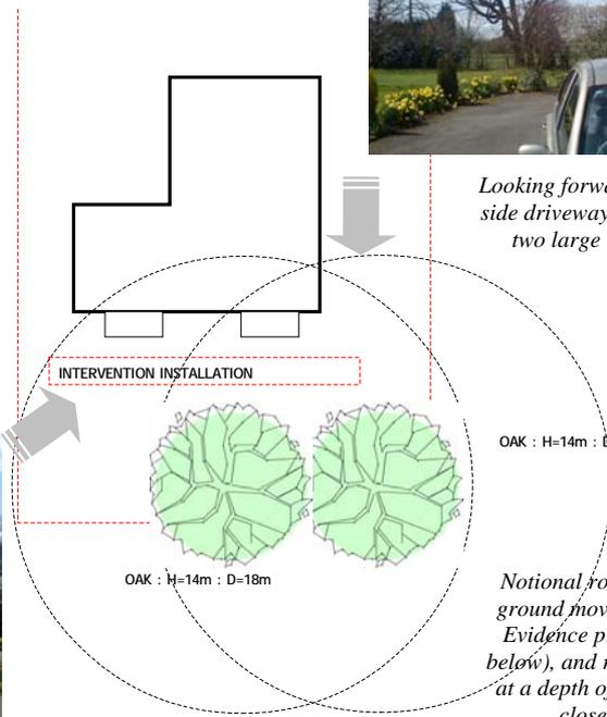
Notional root zones "sufficient to cause ground movement resulting in damage". Evidence provided by soil suctions (see below), and recovering roots from the Oak at a depth of 4mtrs in the boreholes sunk close to the front elevation.
