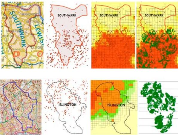
Comparing the claims with the geology serves to illustrate just how important geology is in terms of risk. Southwark have outcropping clay to the south of the Borough, and Islington, to the north. Claim distribution aligns almost exactly.
