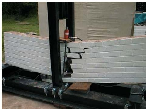
We already have parameters of masonry reinforcement and limiting tensile stresses from the work of Burland, Wroth, Skempton and others, plus the more recent research at the premises of C.P. Bennett in Solihull where masonry panels have been tested to destruction (left).
