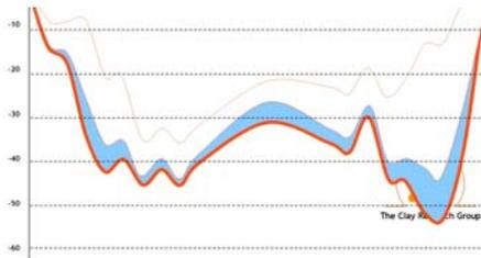
The trees are similar in height to the Aldenham Oak, the ground movement profile from which is shown above, revealing amplified movement at the root periphery.
