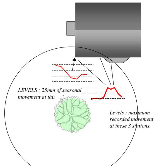
Precise levels confirm movement in the root zone, with maximum of 25mm at the front left hand corner, followed by stations adjoining the bay window.
